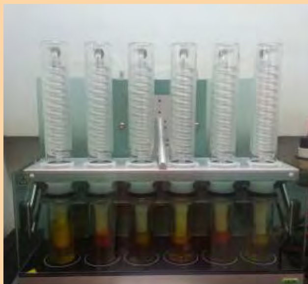
Automated soxhlet extraction system
