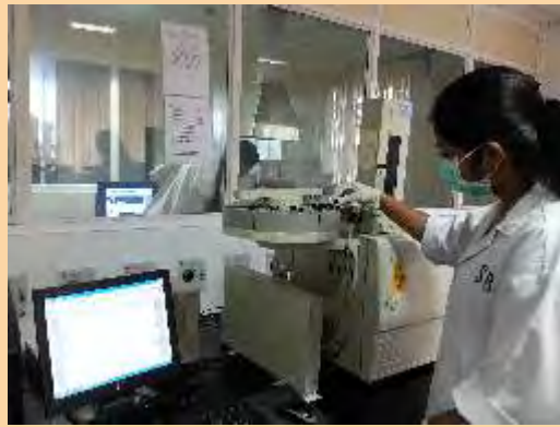
GC with ECD Disulfoton etc are analysed by Gas Chromatograph with FPD.(Flame Photometric Detector)
