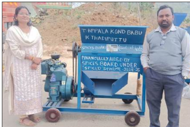
Assistance for installation of pepper thresher at Paderu, Andhra Pradesh
