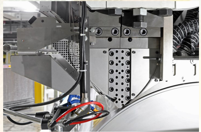
Cloeren Reflex cast film die in touchless configuration.
