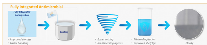
Figure 4. Improved process for fully integrated antimicrobial technology in coatings.
